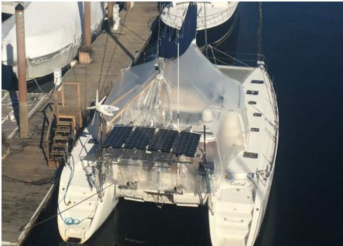
Both solar panels and a wind generator in use for energy.
